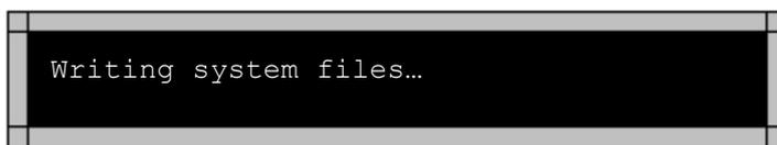
**WARNING:** Do not turn off the power while writing system files. The sign will automatically restart after it finish. Only the JTAG connection is available when the sign is damaged by improper updating operation.
