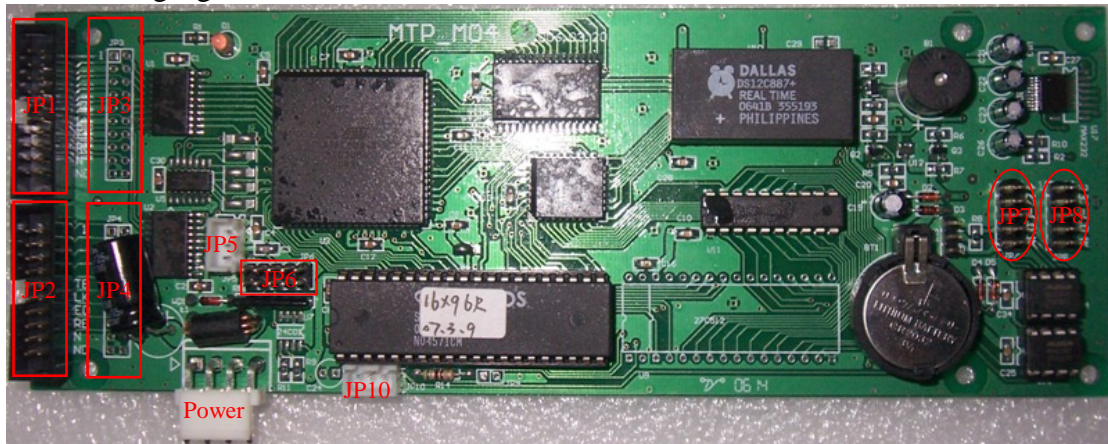
Fig5.3 Control card (MTP_M04)
